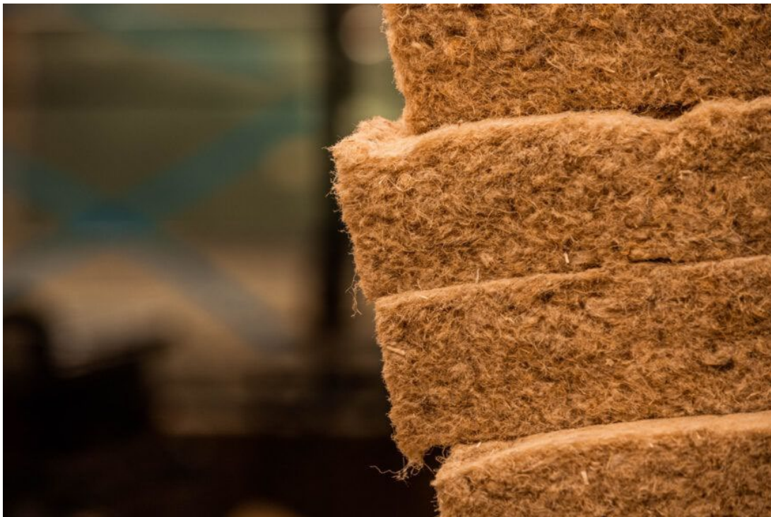
Figure 3: Hempitecture’s HempWool® insulation batts (held by IND HEMP’s team members). These batts are made using airlay thermobonding of hemp fibers, resulting in a high-loft product that fits between wall studs like conventional insulation. The partnership between IND HEMP and Hempitecture delivers a fully domestic, plant-based insulation solution.
