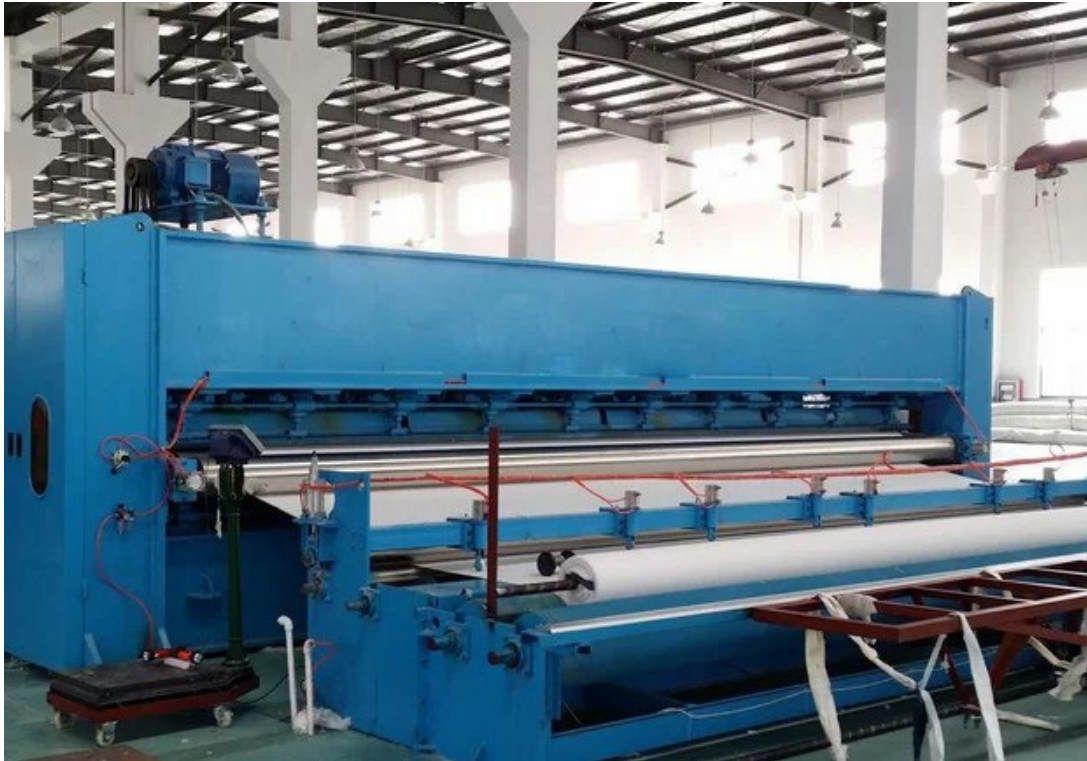
( Needle punching nonwoven process - NWFabric ) Figure 3: A modern needle punch machine (needle loom) in a production line. The blue machine houses the reciprocating needle boards that punch the fiber web as it moves through. Such machines can contain tens of thousands of needles and apply hundreds of punches per minute per needle, depending on design.
