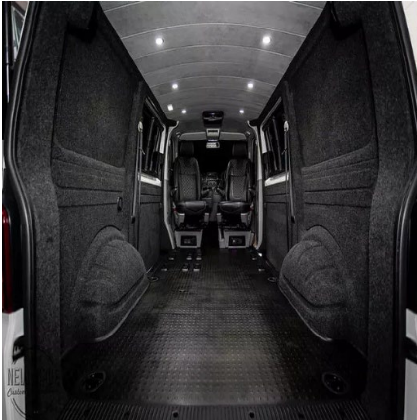
Figure 4. Interior of a vehicle outfitted with needle-punched nonwoven panels for acoustic and thermal insulation.
