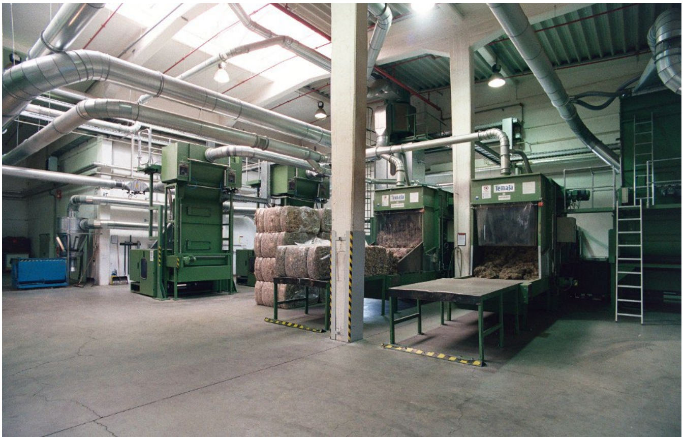
( Mat Production | TWE ) Figure 2: Fiber opening and blending equipment in a needle-punch nonwoven facility. Bales of fiber (right) are fed into opening machines (Temafa openers shown) that loosen and blend the fibers. This prepares a uniform fiber mix (in this case including natural fibers) for the carding or web-forming stage.
